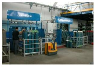
The machine concept ensures very high productivity, more than thirty cylinders per hour with one and only operator managing the whole cycle directly on the control panel. It can be manufactured for 6 cylinders (single bench) or for 6+6 cylinders (DUO version) for additional productivity.
