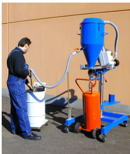
FILLING OF WHEELED FIRE EXTINGUISHER
