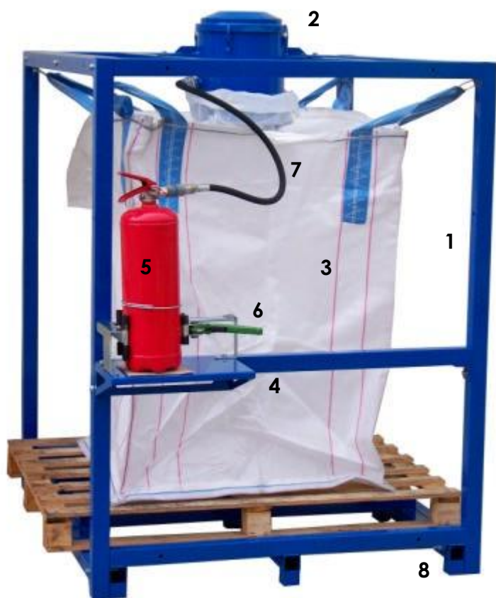
Powder recovery from a pressurized fire extinguisher
